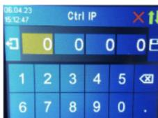
In the case of a control mode with the addition "Manual", the IP address of the signal source must not change during operation (e.g. by a DHCP router), otherwise the AC•THOR or AC•THOR 9s will lose the control signal.
