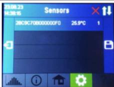
By tapping on the list entry, a number appears at the end of the line. Then the setting must be saved (floppy disc symbol on the right).
