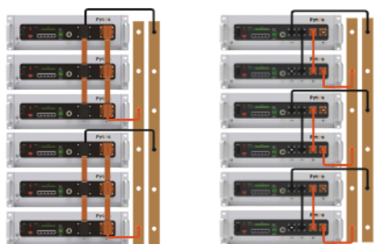
Figure 5-1 Schematic diagram of power cable connection
