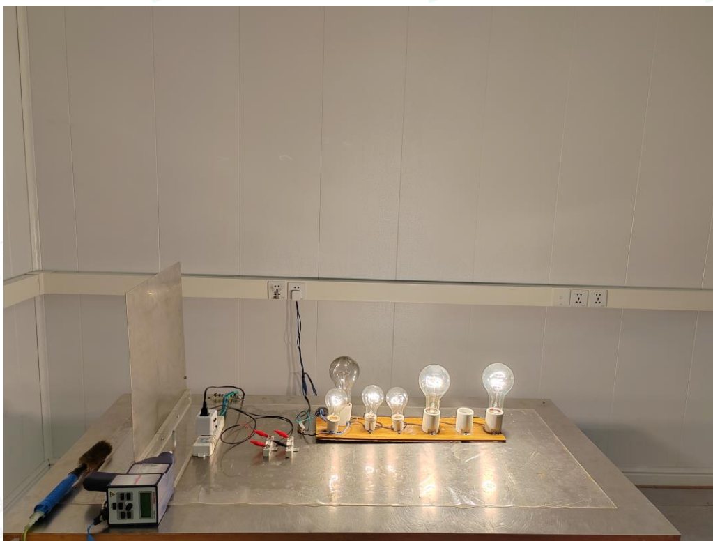
Test Setup Photo of Electrostatic Discharge Test
