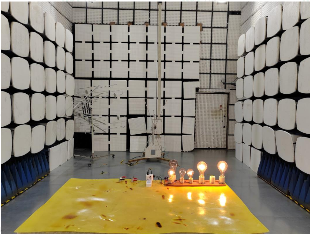
Test Setup Photo of Radiated Measurement (30MHz~1GHz)
